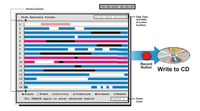
Rotating the **Jog** moves the two arrow cursors across the representation of the recorded video. As the cursors move across the screen the corresponding disk time is indicated in the upper right of the screen. The video representations are color-coded by category. Rotating the **Shuttle** expands (Zooms) the display. The Lowest level (most detail) is indicated on screen with an **(L)**. Pressing the **Enter** button will start Playback from the cursor location.
